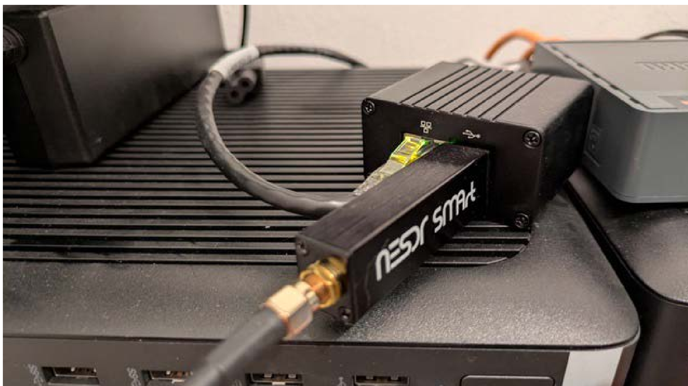
The final implementation — NanoPi with the USB SDR dongle sitting on the firewall.
