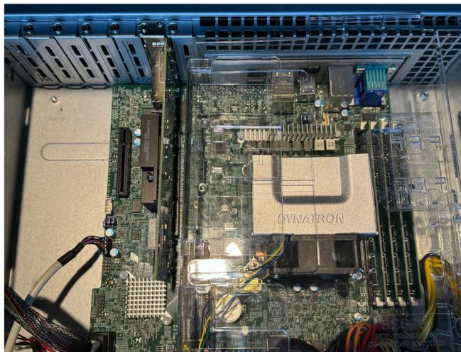
Supermicro X12STH-F Motherboard, CPU PCIe Slot 6 with Intel X710-DA2
