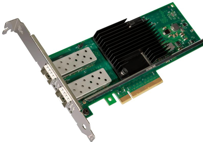
The Intel X710-DA2 PCIe 3.0 Fiber Network Adapter
