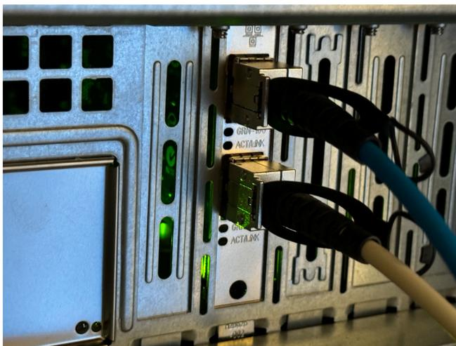
Intel X710-DA2 SFP+ Ports with DAC Cables Attached
