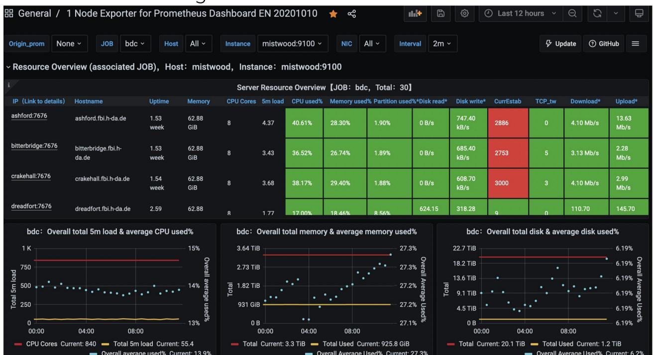
Some of the dashboards can be a bit overwhelming in the amount of data they display at once. I find that an overview dashboard showing me all machines is a good start to see what is going on. When I identify something out of the ordinary, I drill down into that host with an-
