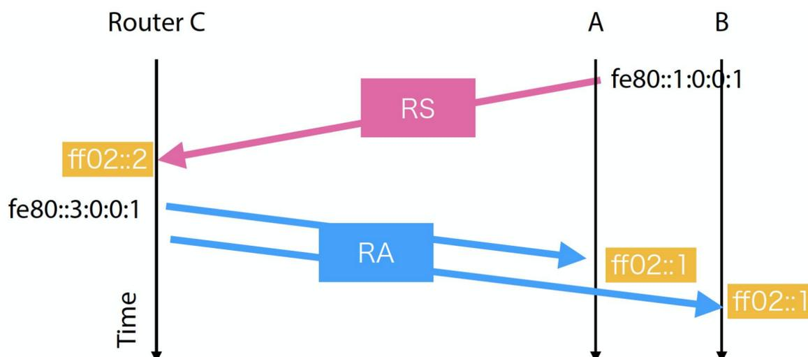
**Figure 4: Timing diagram of Router Solicitation and Router Advertisement**
